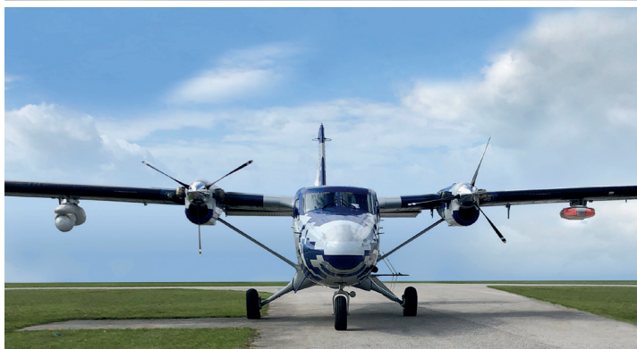
Radar SCAR-Pod with 240° coverage; Guardian 400 Twin Otter with EO/IR and Radar SCAR-Pod
