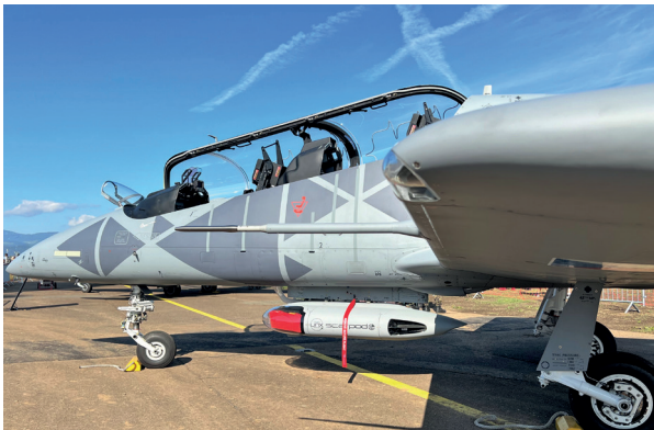
360° Radar-Modular Design; Radar SCAR-Pod on King Air; Radar SCAR-Pod on L39NG
