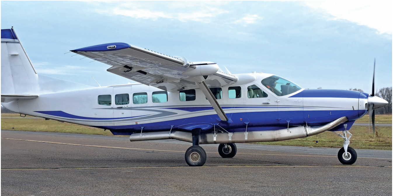
Exhaust Deflector Kit mounted on Cessna 208B CARAVAN
