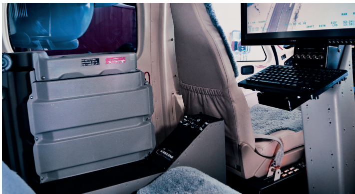
External Camera Lift on AW109; Internal Camera Lift for 10" gimbal
