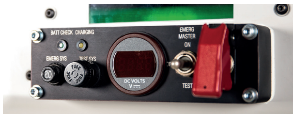
Control Panel for camera lift
