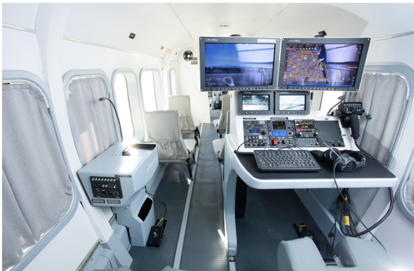
Operator Workstations and Observer Workstation
