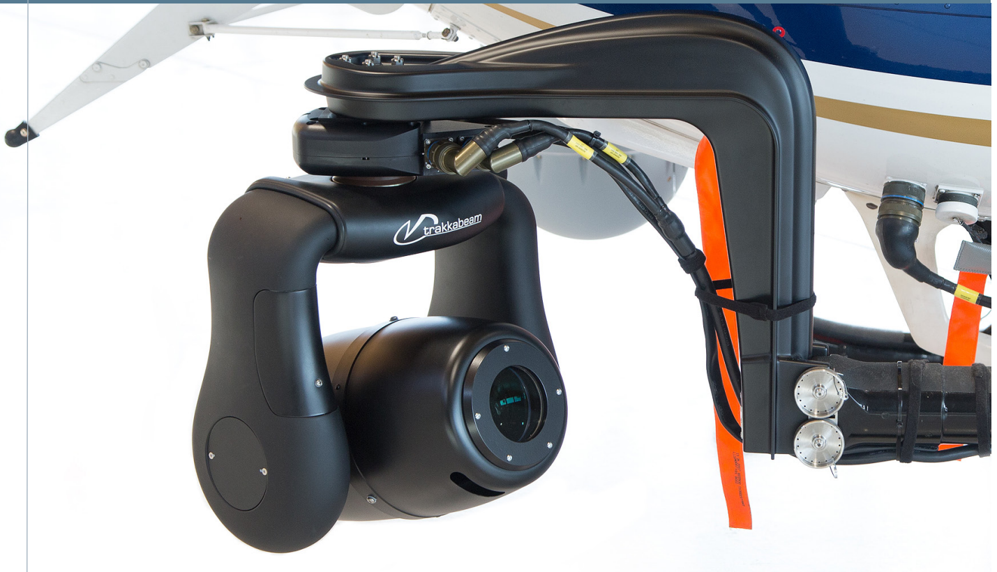
Airbus H 135, Trakka A800 on Searchlight Bracket
