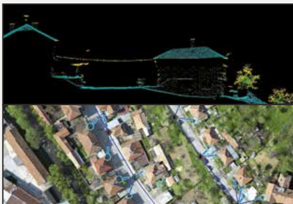
Low voltage power line (3D point cloud + vectorized view)
