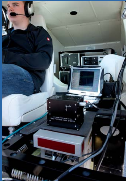
Airborne surveying equipment mounted in multi-mission aircraft (TECNAM MMA)
